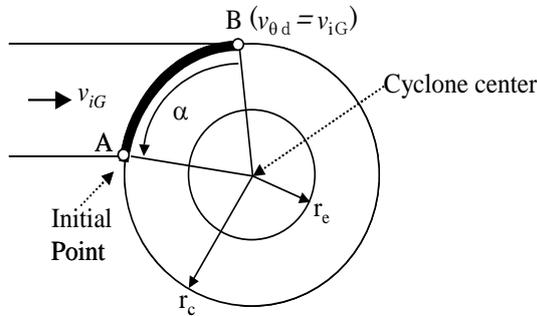
Figure 2. Initial conditions of differential equations inside cyclone.
