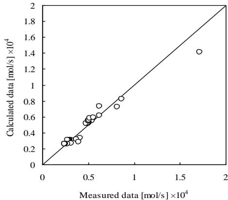
**Figure 5.** Parity plot of experimental CO<sub>2</sub> absorbed flux vs calculated values.
