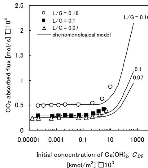
Figure 4. Effect of liquid-gas ratio,  $L/G$ , on  $CO_2$  absorbed flux.
